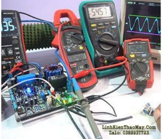
700W Power Output at 90VDC Symmetrical PSU, Signal 1kHz Full video making and test:
