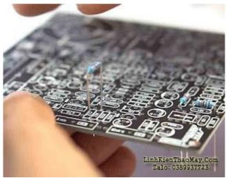
For the PWM Cap freq value I use 220pF multilayer capacitors, dual opamp ICs for Inbal using Low Noise MC33078 SMD op-amps can also use DIP version, dead time resistors use 300 + 39ohm 1 / 4W, comparator uses 2n5551 and C3503 manufacturers ON semi, bat54 diodes using SMD, TR Totem using C2655 and A1020 pairs, for dumper diodes using ES2D or can also use Mur240 or ultrafast 2A diodes, Mosfet using IRFP260N 2 seeds.
