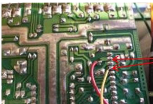
Signal output to amplifier stage
