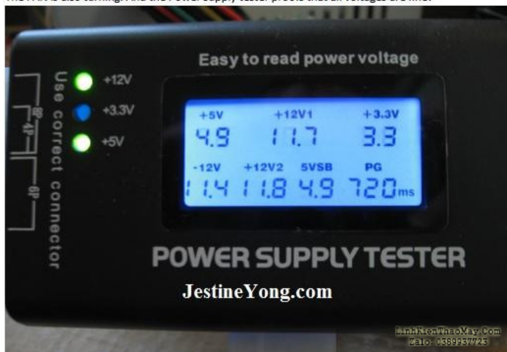
The FAN is also turning. And the Power supply tester proves that all voltages are fine!
