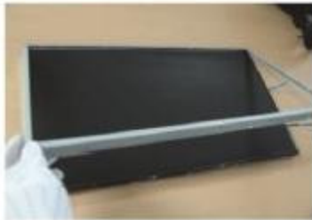
Step7 : Separate case top(push the case top because of damages on COF)
