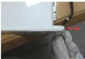
Step13 : Pull the Lamp Ass'y to outside about 10cm using pincette.
