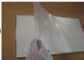
Step11 : remove the Optical Sheets
