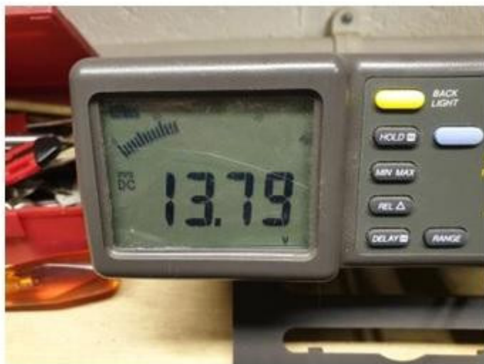
Output voltage remained constant at 13.80v as per manufacturers spec
