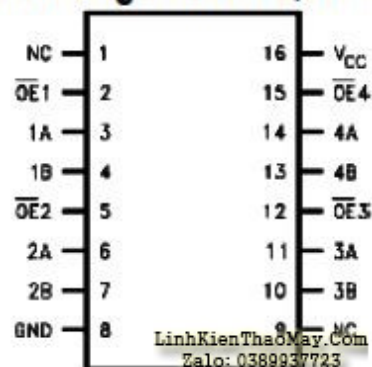
Pin Assignment for QSOP
