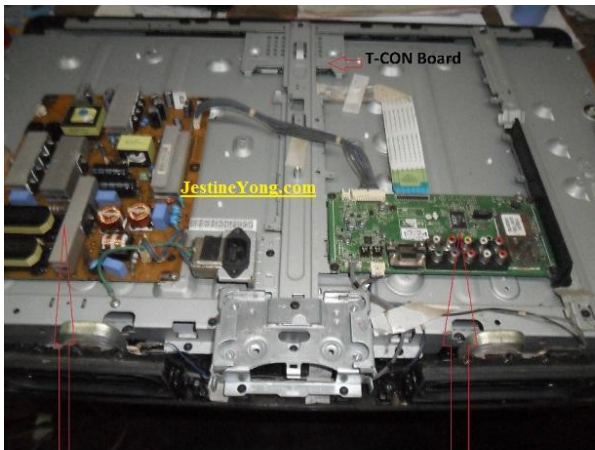
Power Supply and LCD Back light Inverter Board.
