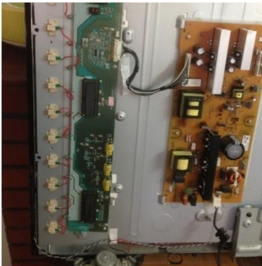
Photo 4-With China backlight inverter board installed
