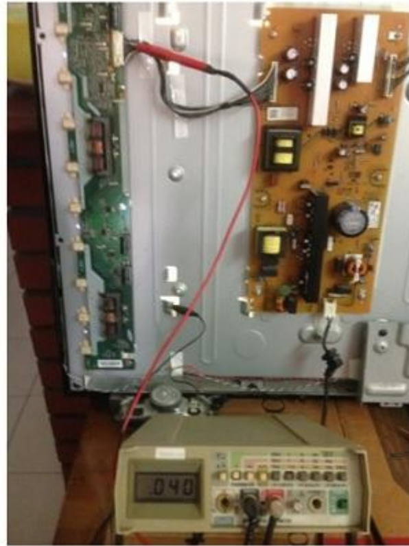
Photo 7: Err Out measured with the transformer swapped.
