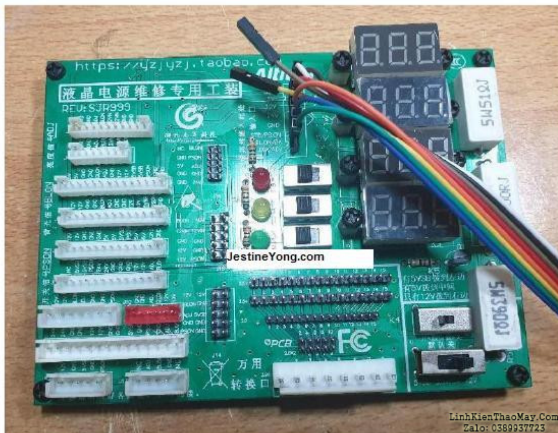
Figure B: PSU Tester
