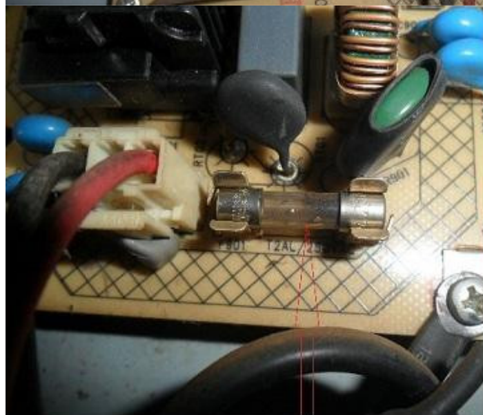
Main Fuse and Power FET is Gone. Defected.
