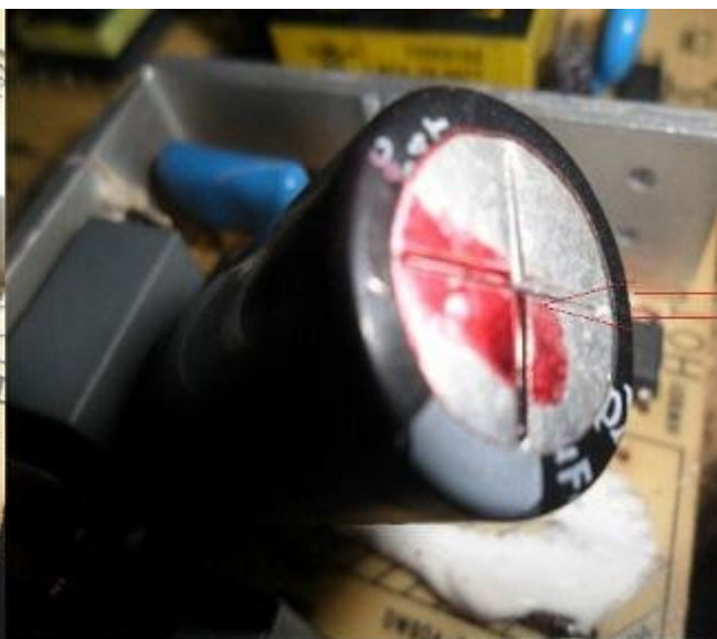
Main Smoothing Cap 400V-120uF Defected
