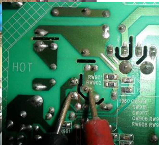
Main Fuse and Power FET is Gone. Defected.
