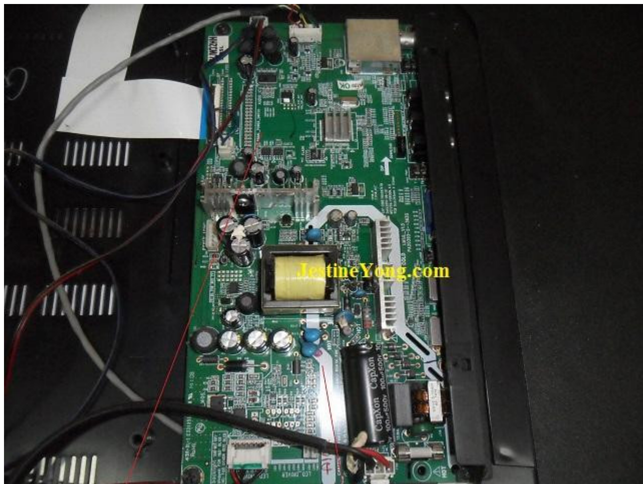
Main Board with Main Power supply Board
